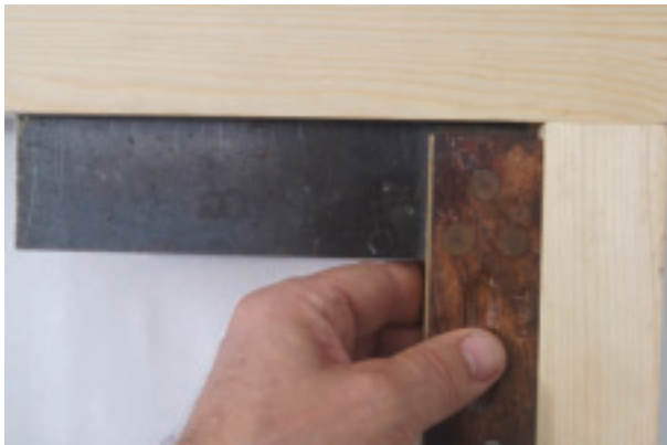
Checking timbers are square to each other
